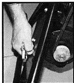
Fig.27: Loosen motor mounting bolts to move motor for further adjustments as needed.
