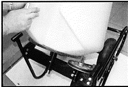
Fig.30: Slide washer onto mixer drum shaft.
